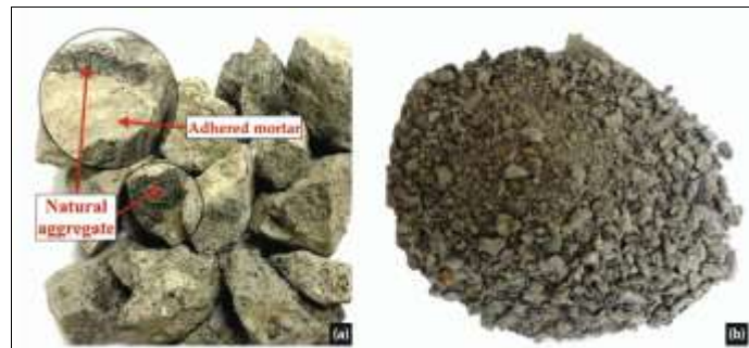
Fig 2: (a) Coarse recycled concrete aggregate (RCA) and AM (b) Fine RCA with ACP
