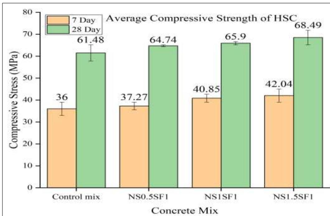
**Fig 5:** Compressive strength test results
