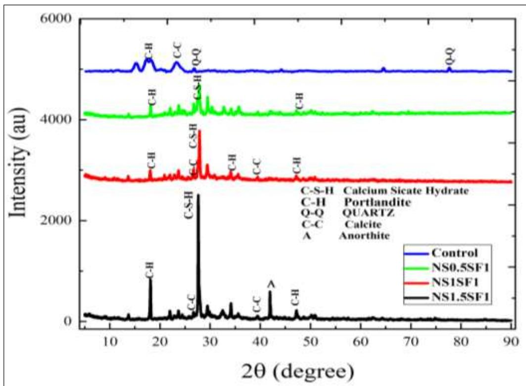
Fig 10: XRD graph of the control sample, NS0.5SF1, NS1SF1, and NS1.5SF1
