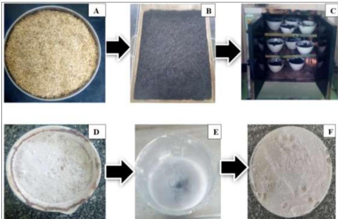
**Fig 1:** A) Rice husk B) Rice husk burned at 400 °C for 3 hours C) Rice husk ash refluxed by HCL(2N) at 70 °C for 1 hour D) RHA heated at 650 °C for 3 hr, E) Nano silica gel, F) Nano silica
