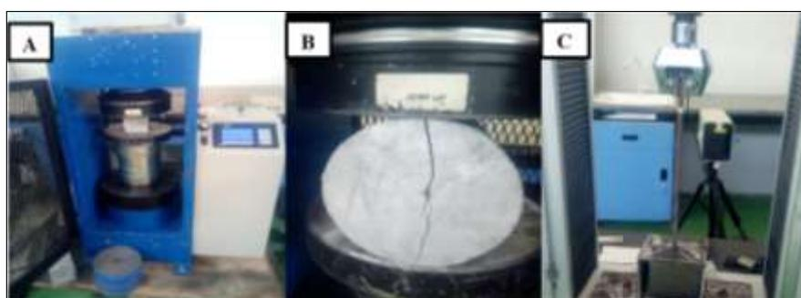
**Fig 7:** Test Set up A) Compressive strength test of Concrete B) Splitting tensile strength test C) Pullout Test
