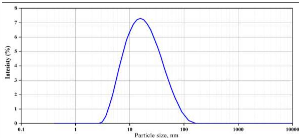
Fig 4: Particle size distributions of nano-silica particles
