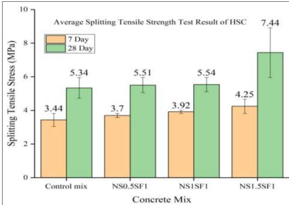
**Fig 6:** Splitting tensile test result
