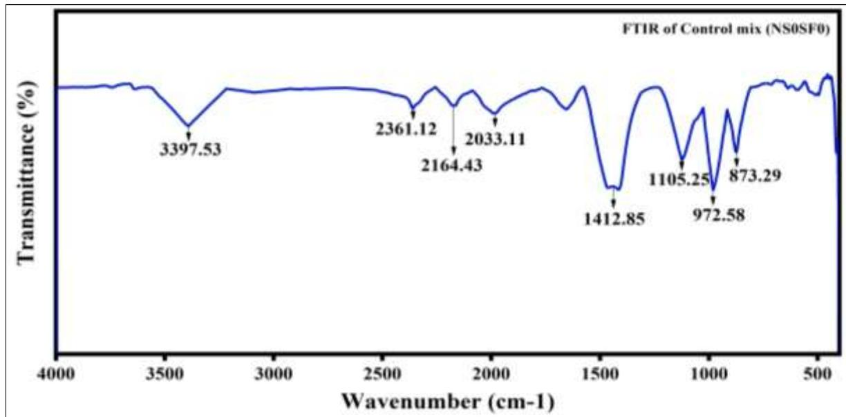
Fig 8: FTIR graph of control sample, NS0SF0
