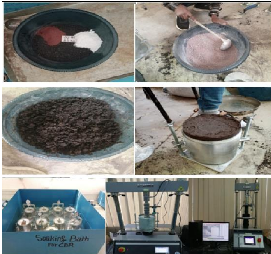
Fig 2: Sample preparation, compaction, CBR and UCS test
