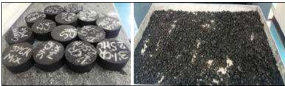
Fig 3: Specimen preparation using Automatic Laboratory Mixer and Superpave Gyratory Compactor
