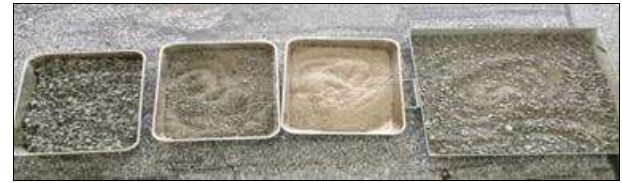
Fig 1: Aggregate from stockpile and blend aggregate prepared in lab
