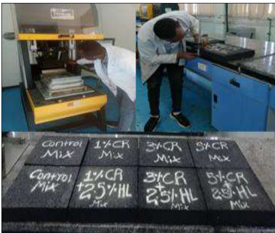
Fig 4: Specimen preparation using Electromechanical Slab Compactor for rutting test
