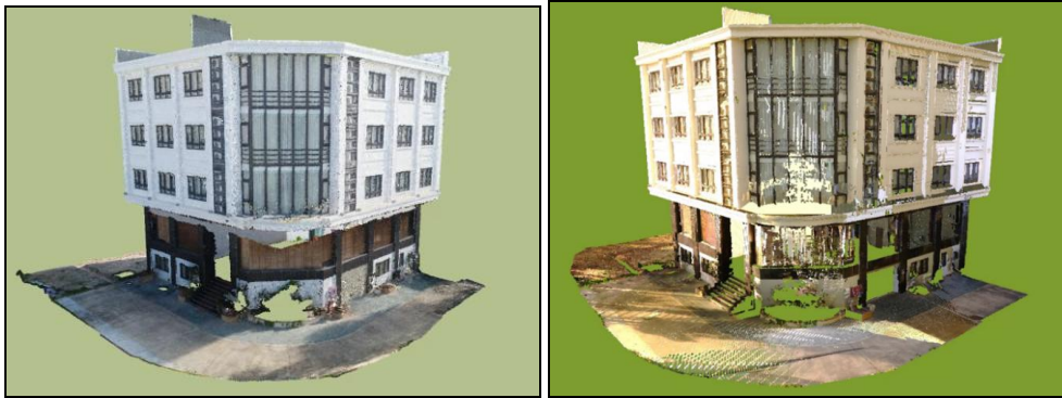
Fig 7: The TLS and UAV-derived point clouds after noise filtering, vegetation removal, and point cloud down sampling
