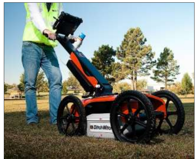
Fig 2(A): Ground penetrating radar in use near Stillwater,
