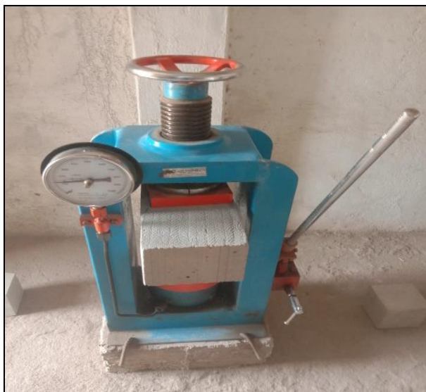
Fig 3: Compressive test on Red Brick and AAC Block
