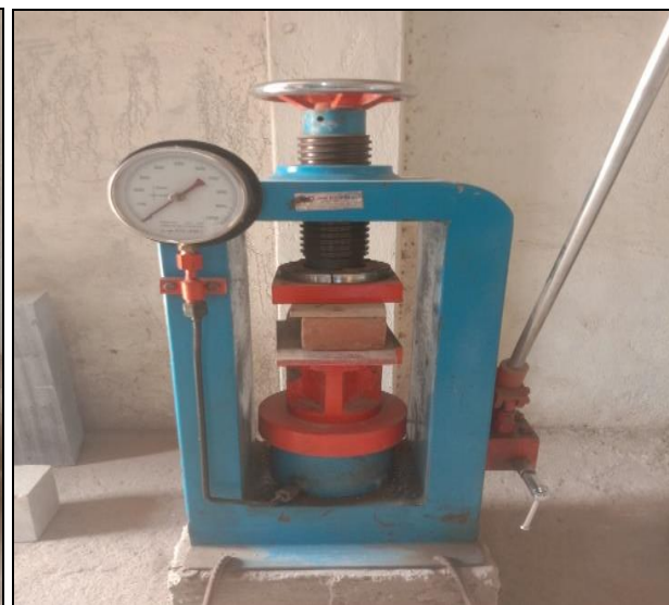
Fig 3: Compressive test on Red Brick and AAC Block
