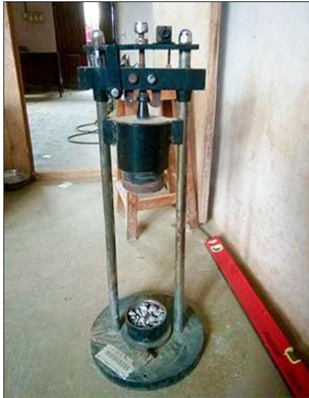
Fig 4: Aggregate impact value test
