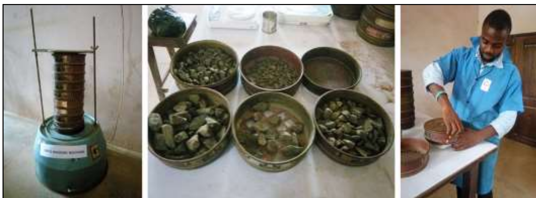
Fig 3: Sieve analysis test
