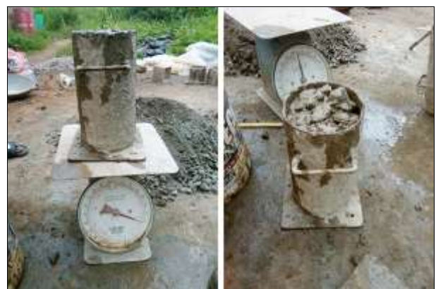
Fig 6: Compacting factor test
