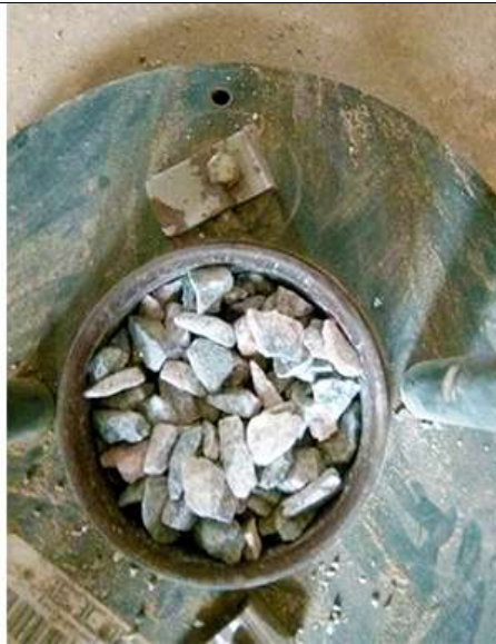
Fig 4: Aggregate impact value test
