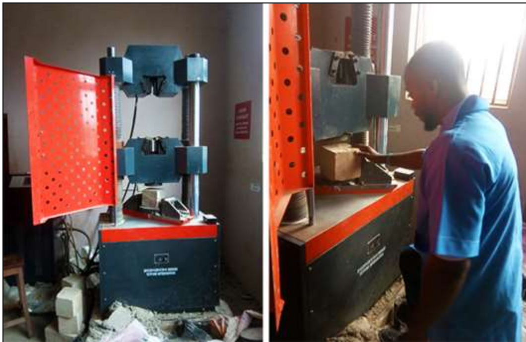
Fig 8: Compressive strength test
