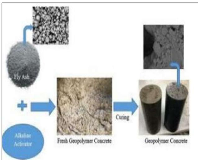
**Fig 2:** Preparation of Geo-Polymer Concrete
