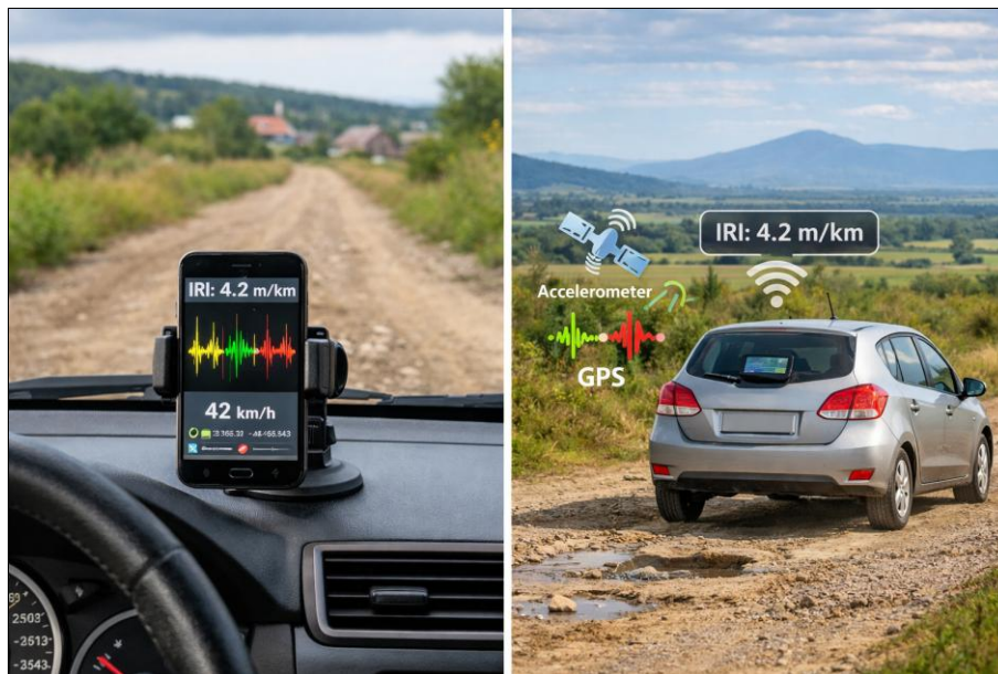
Fig 2: These images depict the process of smartphone-based road road roughness mapping on rural roads, showing a smartphone mounted in a vehicle to measure road roughness and a car driving over uneven terrain for real-time data collection.
