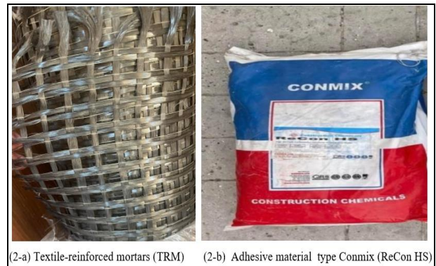
Fig 2: Textile-reinforced mortars (TRM) (2-a), and Adhesive material type Conmix (ReCon HS) (2-b)
