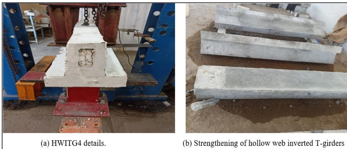
Fig 3: On each side, the beam experiences a common two-point loading scenario (a), while (b) involves the utilization of (TRM) for mechanical reinforcement of hollow web inverted T-girders
