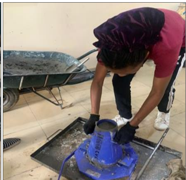
Fig 1: Conduction of slump test
