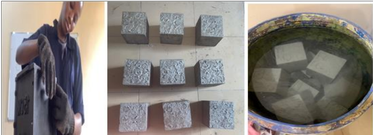
Fig 2: Demolding, sampling and curing of concrete cubes
