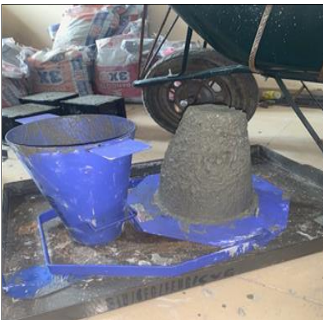
Fig 1: Conduction of slump test
